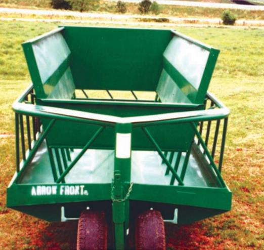
Inserts are at an angle that allows feed to flow down without bridging and resists overflowing. **Adjustable height** of the inserts control the feed-flow of different types of feed. Inserts are removable when feeding round bales, to allow cattle to get at the total bale. Manger depth is ideal to prevent overflow and eliminate residual spoilage. 12 gauge rust resistant steel feed manger. **Rust and acid resistant green paint.**
